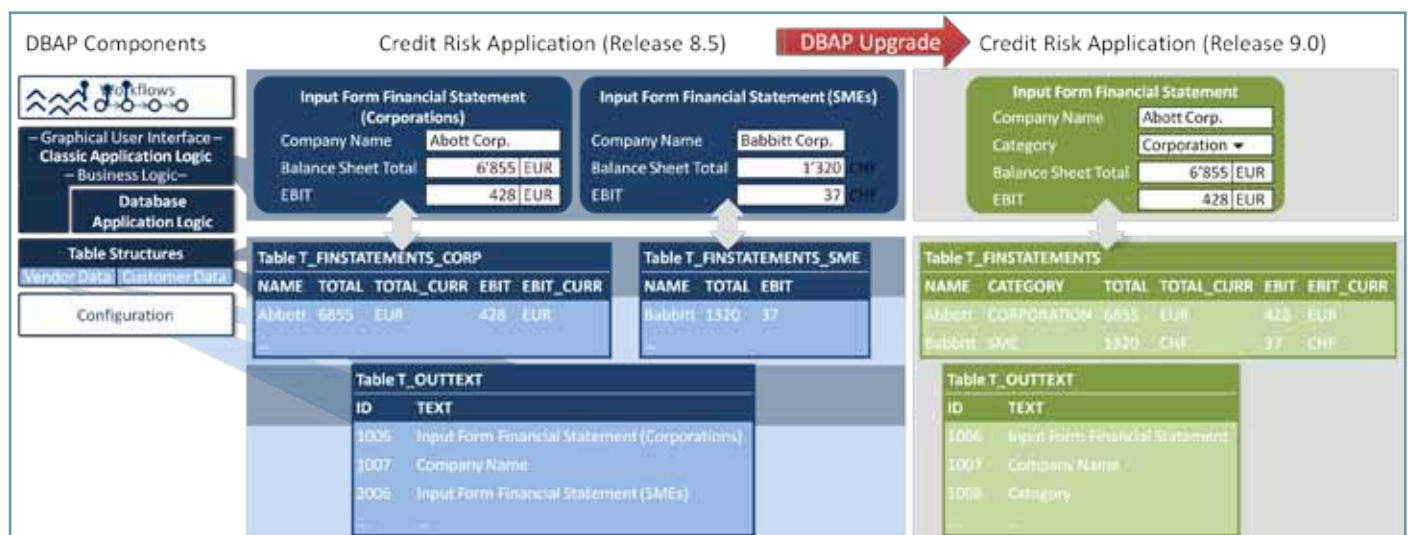
Figure 1: DBAP components (left) and sample application (release 8.5 - middle - and release 9.0 - right) with GUI (upper part) and financial statement input forms (middle and right, upper part) and corresponding database tables (lower part).
